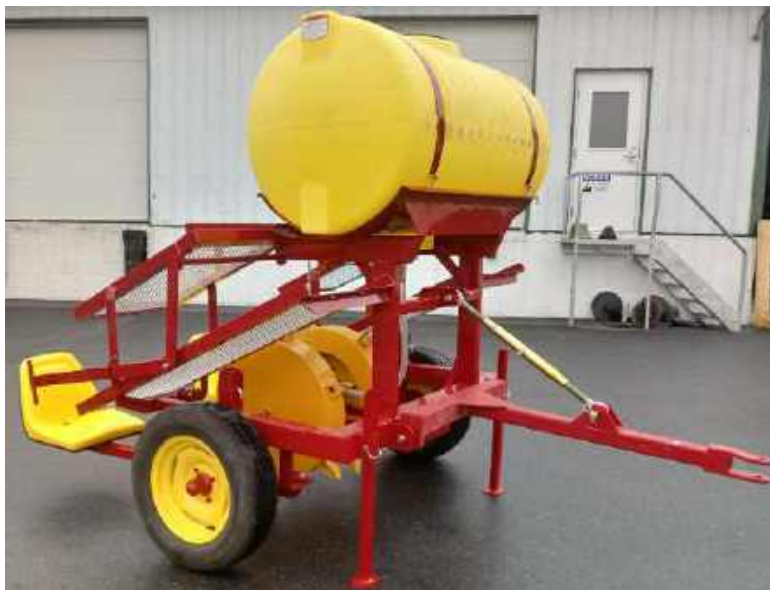
Model P1500 Combination Pull-type with large transport wheels, It converts easily to 3-point hookup by pulling 3 pins & dropping the hitch. Has an adjustable turnbuckle on hitch for easy leveling. Used tires with new rims. Steel wheels optional. 150 gallon tank. $ 3390.00
