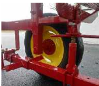
Model P1500 Combination Pull-type with large transport wheels, It converts easily to 3-point hookup by pulling 3 pins & dropping the hitch. Has an adjustable turnbuckle on hitch for easy leveling. Used tires with new rims. Steel wheels optional. 150 gallon tank. $ 3390.00
