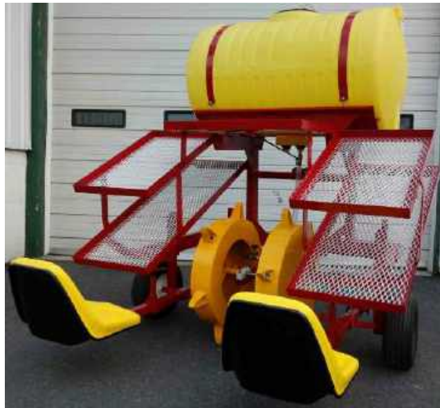
Model P150 3-point Hookup 3pt allows for tighter turn radius at the end of the row. Cat 1 & 2 lift pins, Requires tractor with lift capacity of almost 3000 lbs. 40-80 hp, 4wd or loader helps, 150 gal. tank. $ 2900.00
